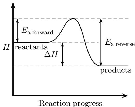
$E_a$  for the forward reaction = 40 kJ/mol, so  $E_a$  for the reverse reaction = 100 kJ/mol.
