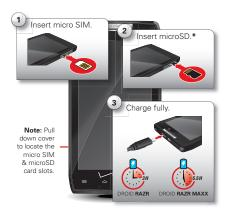
Optional. A microSD memory card is pre-installed in Motorola XT912, XT912M, and XT912W models. For other models, you can purchase a microSD card separately, if desired.
